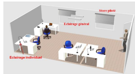
Living lab – smart lighting
